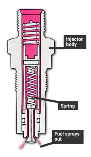
Two main types of injector can be fitted, depending on whether the
