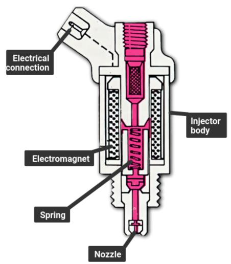
The injector in an electronic system is also held closed by a spring, but is opened by an electromagnet built into the injector body. The electronic control unit determines how long the injector stays open.
