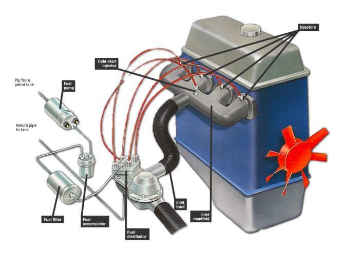
Petrol-engined cars use indirect fuel injection. A fuel pump sends the petrol to the engine bay, and it is then injected into the inlet manifold by an injector. There is either a separate injector for each cylinder or one or two injectors into the inlet manifold.
